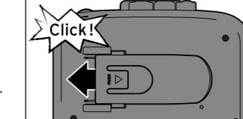
Slide the transport clip into the runners as far as it will go. You should hear and feel the transport clip click into place.
