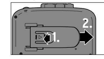
Pull the (PUSH) catch on the transport clip to open it (1.) and pull the transport clip sideways to remove it (2.).
